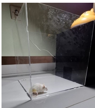
Figure 3. Light Dark Box Apparatus.
