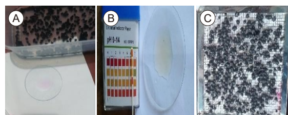
Figure 3. (a) Chitosan–biochar–urea–Fe beads in an alkaline state (basic), showing their initial formation; (b) Beads that have been neutralized; (c) Beads after washing to achieve neutral pH.
